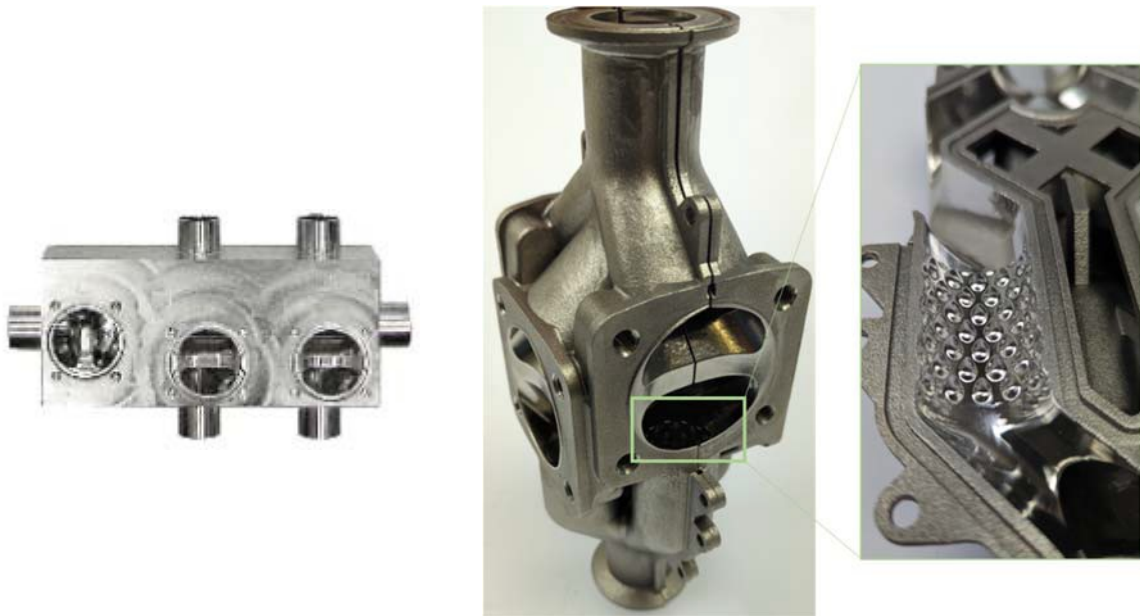
Figure 1: Milled and conventional valve block (left) and valve assembly optimised for the LPBF process as HygAM demonstrator (middle and right). The inner channel geometry has a curved structure for improved cleanability.
