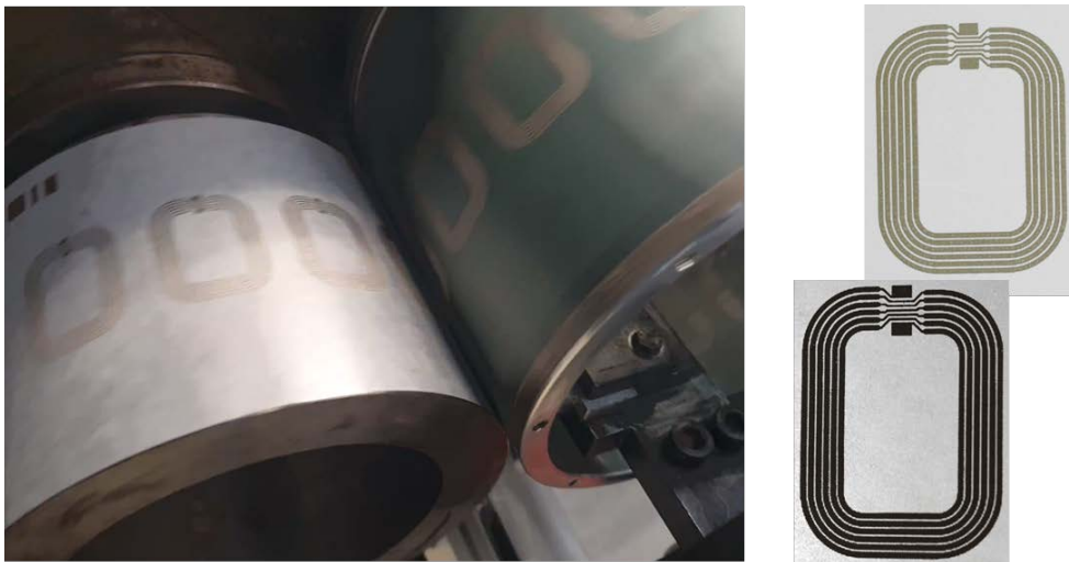
Figure 4: Roll-to-roll screen printing process using the example of printed RFID antennas (Source: TU Chemnitz)
