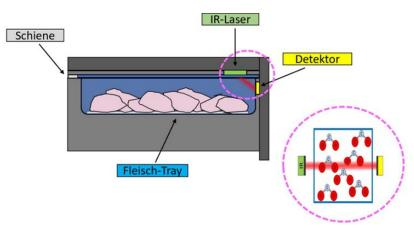
Figure 1: Schematic representation of the measuring device for non-invasive CO<sub>2</sub> determination in the MIR range.
