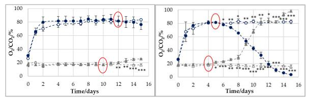
Figure 4: Development of  $O_2$  ( $\circ/\bullet$ ) and  $CO_2$  ( $\Delta/\blacktriangle$ ) in the packaging headspace with ( $\bullet/\blacktriangle$ ) and without poultry ( $\circ/\Delta$ ) at an initial gas concentration of 80%  $O_2/20\% CO_2$  stored at 4°C (left) and 10°C (right). The indices show a significant difference between the curves with and without meat (\* P < 0.05, \*\* P < 0.01, and \*\*\* P < 0.001).
